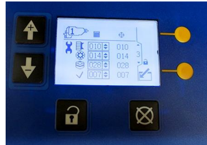
Set up screen for maintenance totalizer 10
